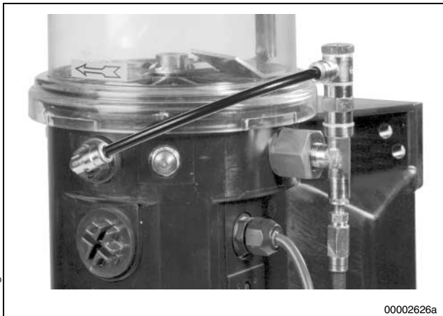
Fig. 15 Pressure relief valve with grease return
